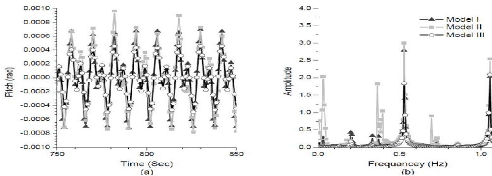
**Figure 14: Responses under Regular Waves, WHA=0° A) Time History, B) Power Spectrum Density**
