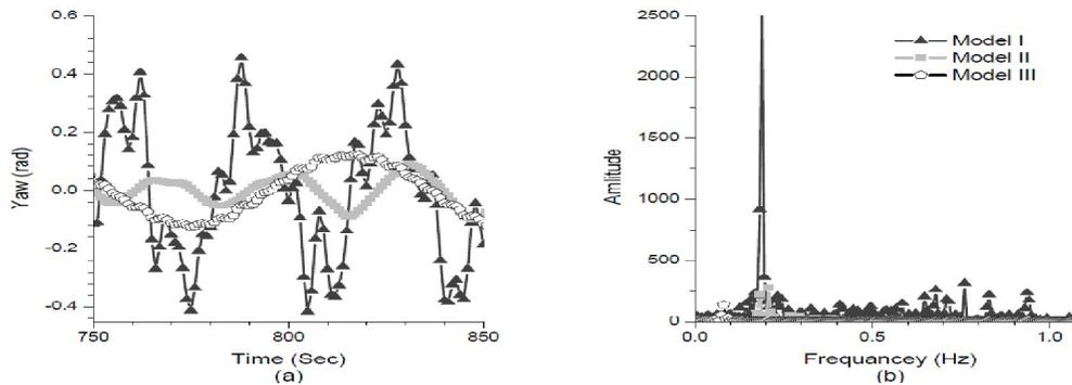
Figure 16: Responses under Random Waves,  $WHA=90^\circ$  A) Time History, B) Power Spectrum Density
