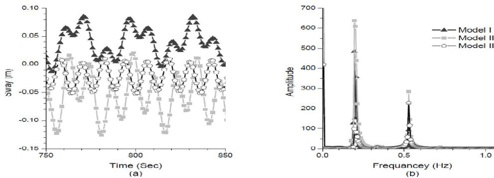
Figure 12: Responses under Regular Waves, WHA=0<sup>0</sup> A) Time History, B) Power Spectrum Density
