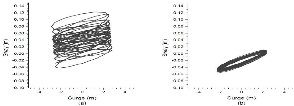
Figure 11: Instability Plane for Surge-Sway (WHA=0<sup>0</sup>) A) Model I, B) Model III
