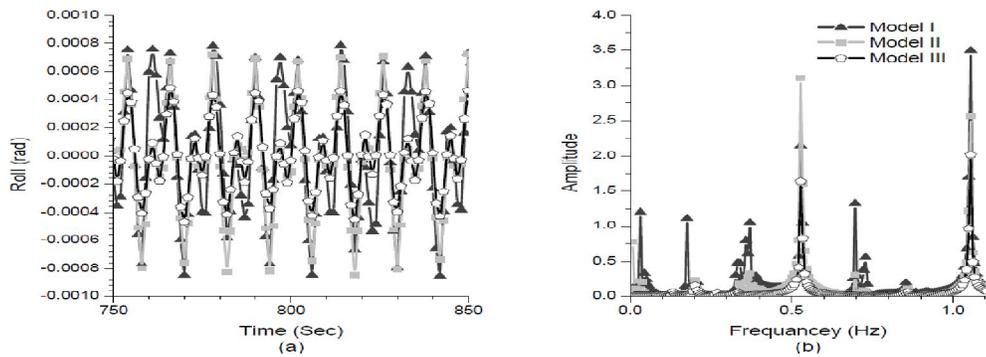
**Figure 13: Responses under Regular Waves, WHA=90° A) Time History, B) Power Spectrum Density**
