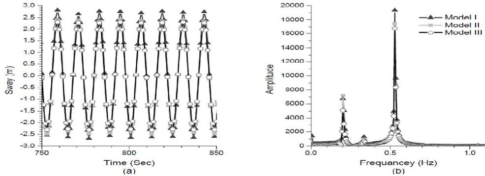
Figure 9: Responses under Regular Waves, WHA=90<sup>0</sup> A) Time History, B) Power Spectrum Density
