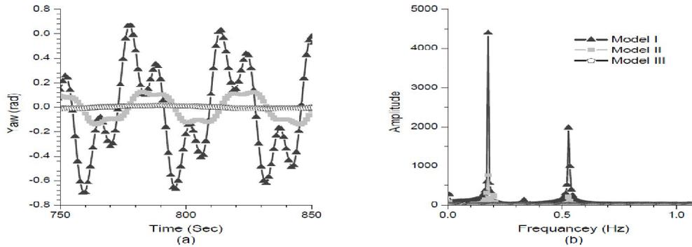
Figure 15: Responses under Regular Waves,  $WHA=90^\circ$  A) Time History, B) Power Spectrum Density
