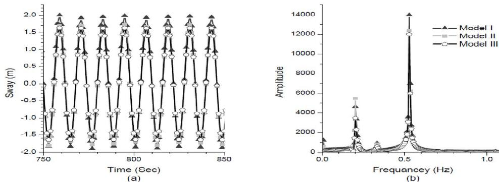
Figure 8: Responses under Regular Waves, WHA=45° A) Time History, B) Power Spectrum Density
