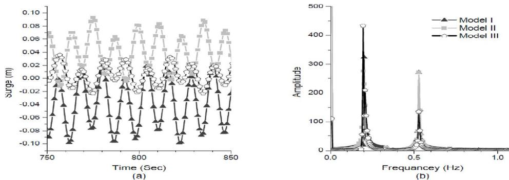
Figure 5: Responses under Regular Waves, WHA=90° A) Time History, B) Power Spectrum Density
