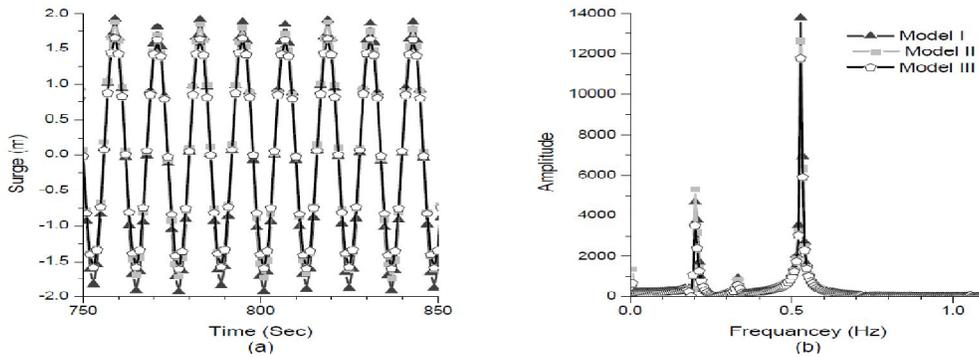
Figure 4: Responses under Regular Waves, WHA=45° A) Time History, B) Power Spectrum Density
