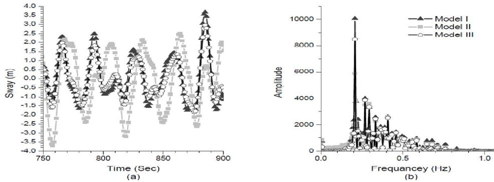
Figure 10: Responses under Random Waves, WHA=90<sup>0</sup> A) Time History, B) Power Spectrum Density
