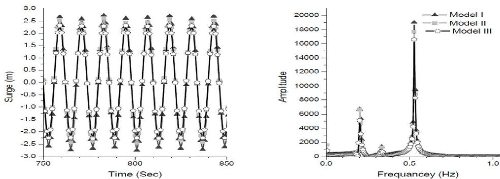
Figure 2: Responses under Regular Waves, WHA= $0^\circ$  A) Time History, B) Power Spectrum Density
