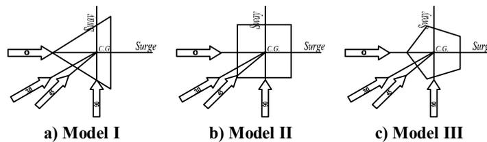
Figure 1: Multi-Directional Waves in Degrees
